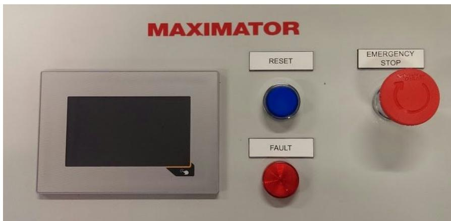
The operator controls include the HMI (Human-Machine Interface), emergency stop, reset button, and fault lamp.
