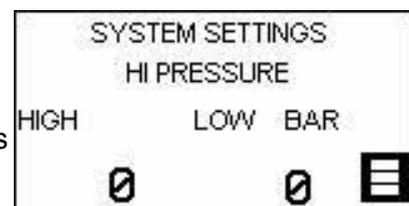
The maximum compressor stop pressure (HI) is normally 350 Bar, and the minimum for this value is normally 150 Bar. The control system will not allow values outside the preset range to be entered.
