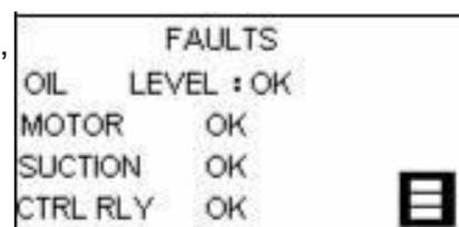
To acknowledge the alarm and reset the control system to allow the compressor to run again, you must press the 'RESET' key. If the alarm condition is no longer present, the red alarm lamp will go out, and it will be possible to restart the compressor.
